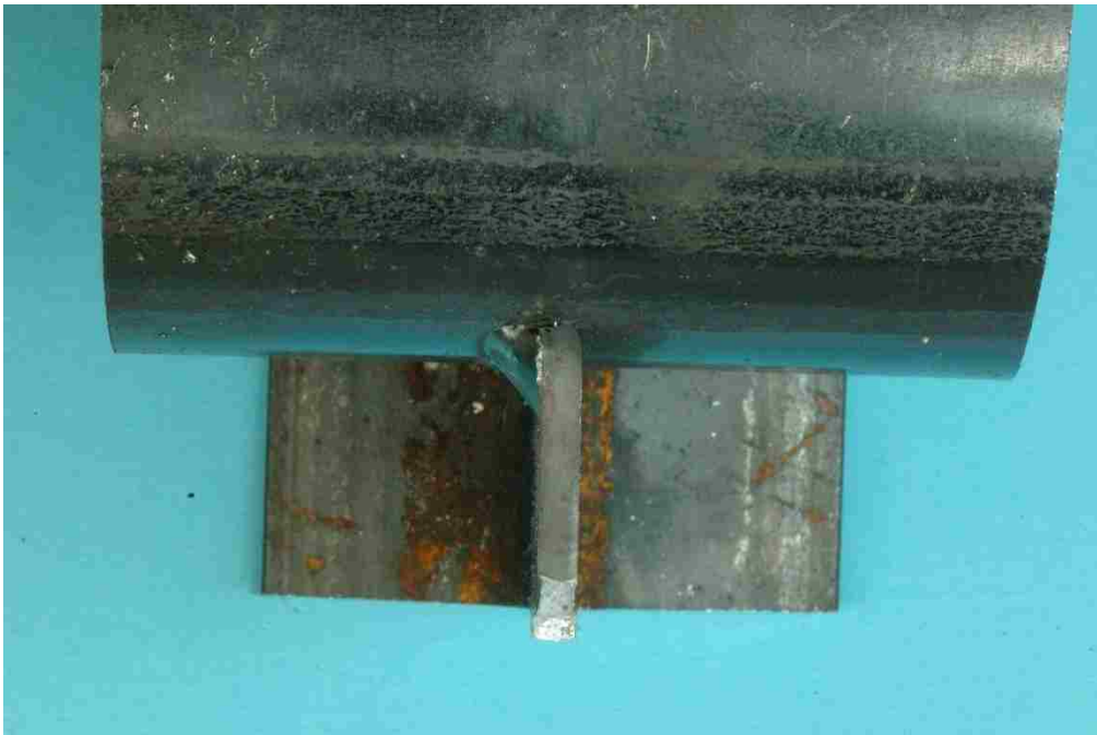
Figure 77. S5-T2 west crack plane, bottom half
