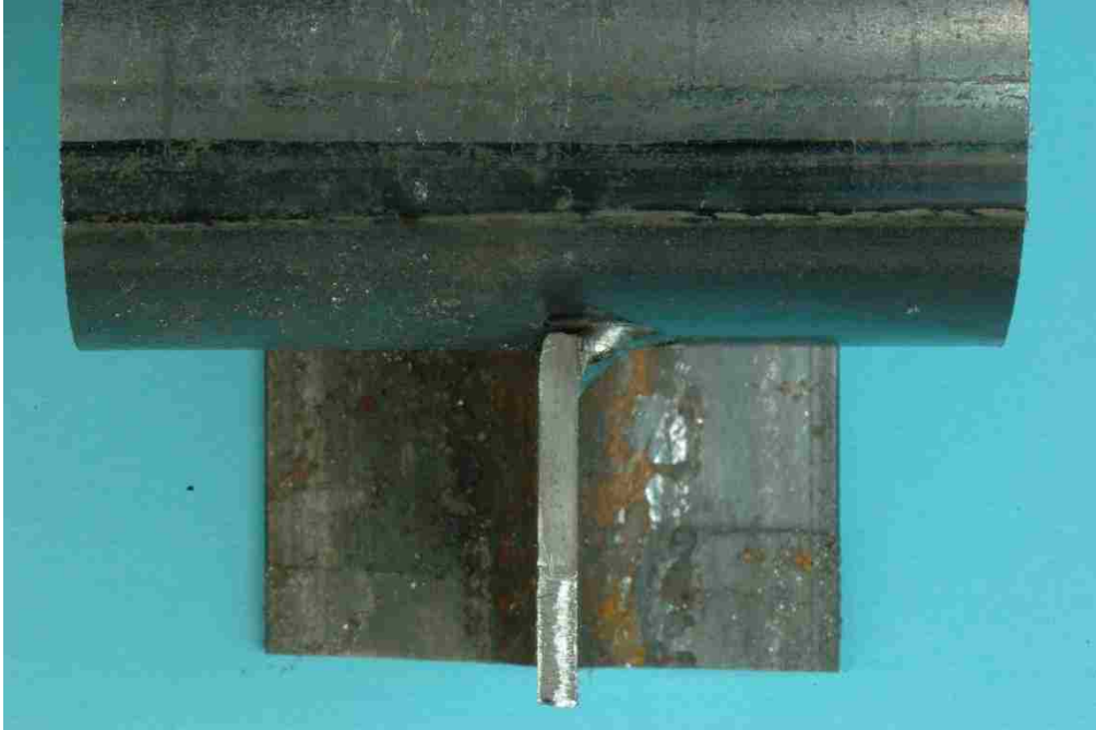
Figure 76. S5-T2 east crack plane, bottom half
