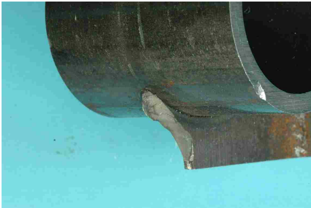
Figure 79. S9-T2 west crack plane, bottom half
